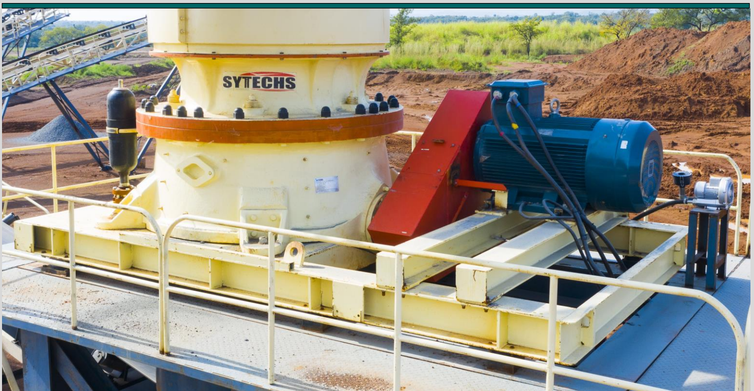
Skid mounted Unit. The cone crusher along with the driving electric motor are both mounted on a skid structure to reduce vibration and belt hammering. This results in better driving performance and longer motor bearing/counter shaft bushing life.
